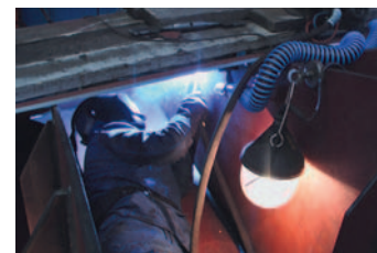
Welding smoke extraction in shipyards
