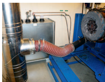
Diversion of engine exhaust gases to dynamic power analysers
