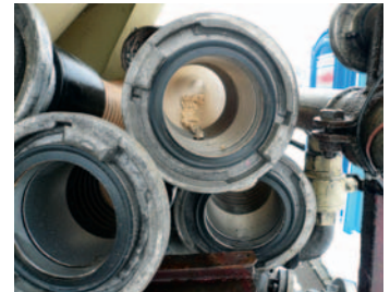
Adaptor for Pellet delivery through silo vehicles
