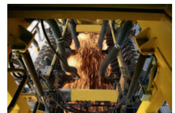
Abrasive dust extraction in rail vehicles
