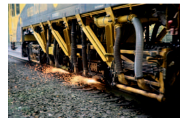
Abrasive dust extraction in rail vehicles
