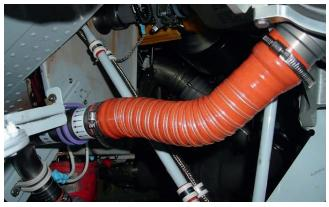
Electrically conductive vent hose in an aircraft tank system, which also diverts electrostatic charging
